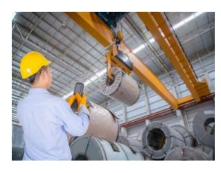
Operators must know the load capacity of their shop crane. Loads that exceed the limits of the crane should not be moved. The load rigging requirements need special attention. Loads that cannot be safely rigged should not be lifted. Before moving loads, the crane operator should inspect the path of the crane for obstacles and people; the path must be clear before starting any crane movements.
