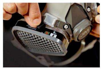
The ESLI is an area on the cartridge that changes color when it's time to replace the cartridge.
