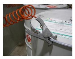
If the static electricity builds up and can't find its way to the ground, it discharges as a spark. Usually, the spark goes unnoticed. But in the presence of some substances and in certain atmospheres, it can set off an explosion.
